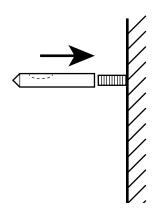
• Unscrew Part C into 2 pieces. Hold the larger part in the WC, insert the threaded part from the outside and tighten using part E. Ensure that the smaller, metal thread is pointing vertically upwards
