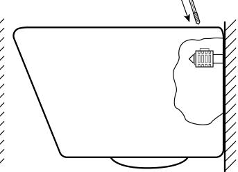
• Slide the WC onto the steel pegs
